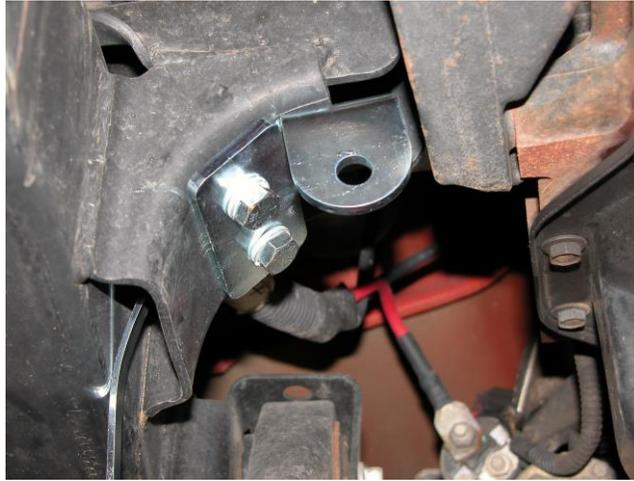
**Step 3:** Repeat steps 1 and 2 on the passenger side motor mount. On the passenger side, the T-shaped nut plate is more easily inserted from the bottom of the motor mount as shown above. The view above is from the front.
