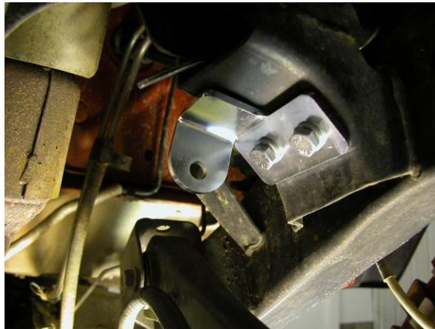
**Step 2:** Take the mounting bracket and attach it to the bottom of the motor mount using two of the 3/8-16 bolts with lock washers with the tab to the rear of the vehicle. The view in the picture above is looking from the front. **NOTE: On the driver side, the tab MUST be to the rear of the vehicle.**
