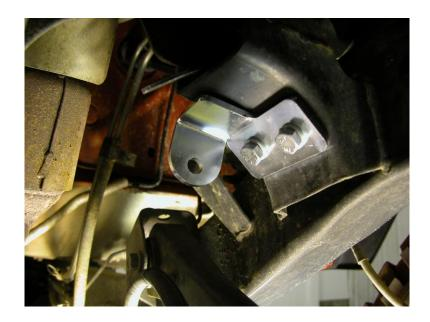
**Step 4:** Take the mounting bracket and attach it to the bottom of the motor mount using two of the 3/8-16 bolts with lock washers with the tab to the rear of the vehicle. The view in the picture above is looking from the front. **NOTE: The tab MUST be to the rear of the vehicle or control arm damage could result.**
