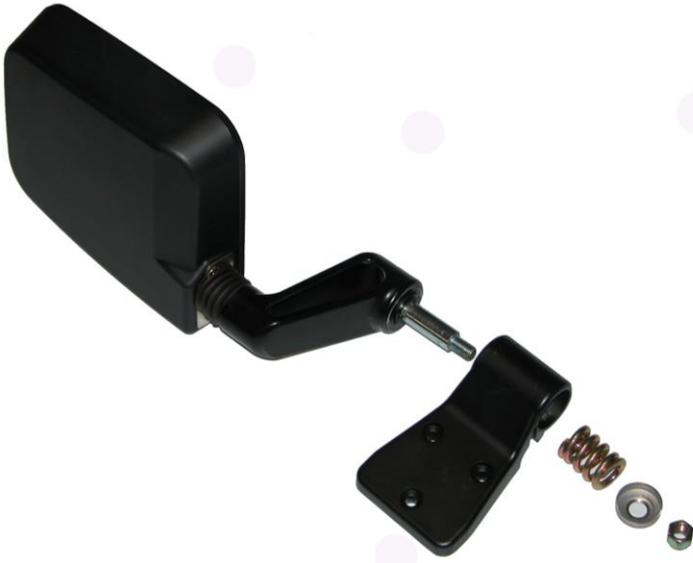
**Step 4:** Mount the mirror into the new relocation bracket using the cup washer and nut. Position the mirror and tighten the nut.
