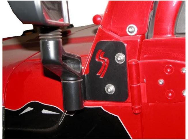
**Step 3:** Disassemble the mirror from the original mirror mounting bracket saving the nut and "cup" washer to be re-used. The parts will look like the picture below. The "cup" washer can be replaced with a standard flat washer if necessary.
