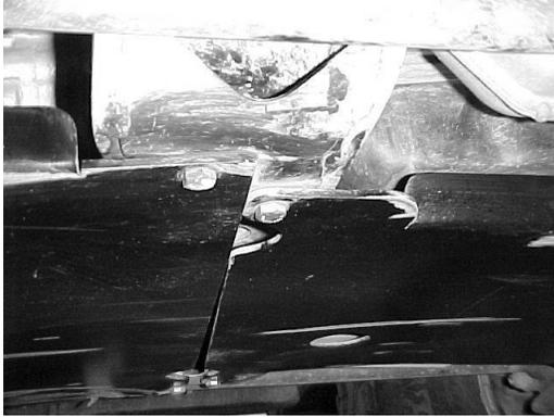
**Step 5:** At this point the skid plate should be loosely attached at the front. Using two of the 5/16x 1.0” bolts, nuts, and lock washers, bolt the rear of the skid plate and transmission cross-member together. If one of the holes does not line up properly, tighten the bolts that are installed and use the hole in the skid plate as a guide to drill a new hole in the cross-member. However, you should be able to get both holes lined up by simply moving the plate a little.
