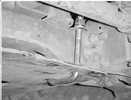
**Step 3:** Take the u-bolts that are provided and place them through the holes towards the front of the skid plate. The left photo is the passenger side and the right photo is the driver's side when viewed from the front of the vehicle.
