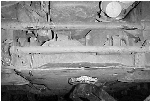
**Step 2:** Position the engine/transmission skid plate under the vehicle so that the leading edge of the skid plate is facing forward. The leading edge has three nuts welded in place to its top surface. Place the skid plate on a floor jack and raise it so that the leading edge of the skid plate extends a little forward of the cross-member that supports the front differential.
