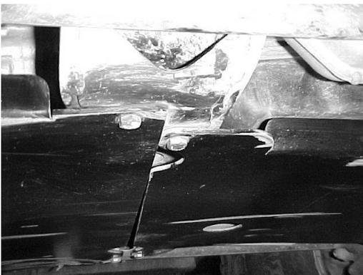
**Step 3:** At the front of the transfer case skid plate install the two 5/16 x 1.0" bolts, nuts and lock washers through the holes in the transmission cross-member.
