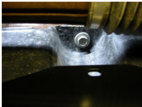
**Step 7:** The 7" Mounting Bracket with Nut is installed at the rear, inboard side of the skid plate. Remove the factory mounting bolt that is above the slotted hole. Place the bracket in position and install one of the 3/8-16 x 1" Hex Head Bolts, a flat washer, and a lock washer through the skid plate into the nut on the bracket. Then re-install the factory mounting bolt.
