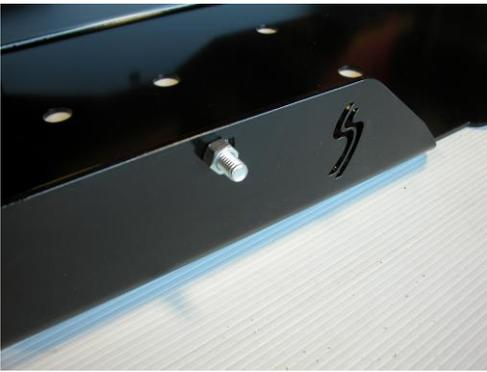
**Step 3:** Place five of the carriage bolts through the holes on the side of the skid plate with the Skid Row logo cut out as shown in the photo at left. Their threads should face outward. Put a nut on each one to keep it in place while positioning the skid plate.
