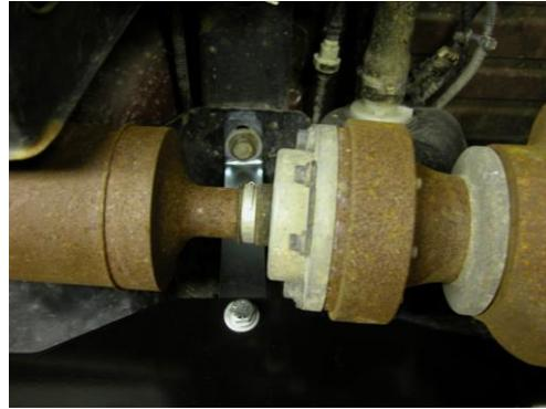
**Step 8:** The Mounting Bracket w/o Nut is installed at the rear, outboard side of the skid plate, near the Skid Row logo. Again, remove the factory skid plate mounting bolt from the chassis. Then remove the nut that was installed on the carriage bolt. Place the bracket over the carriage bolt and install the flat washer, lock washer, and nut. Then re-install the factory mounting bolt through the bracket as shown.
