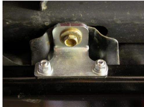
**Step 6:** The 6" Mounting Bracket with Nut is installed in the middle, inboard side of the skid plate, near the accordion seal on the driveshaft. Remove the factory mounting bolt that is shown in the photo below. Place the bracket in position and install one of the 3/8-16 x 1" Hex Head Bolts, a flat washer, and a lock washer through the skid plate into the nut on the bracket. Then re-install the factory mounting bolt.
