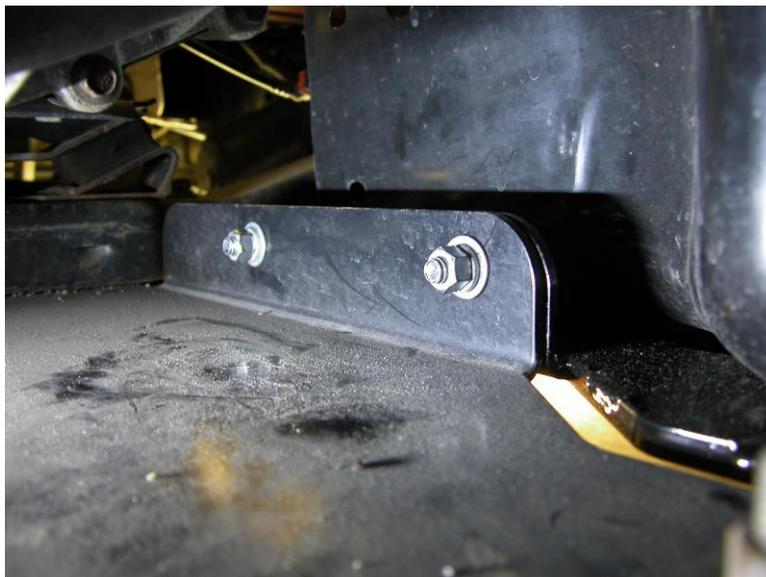
**Step 10:** Re-install the factory mounting bolt for the transfer case skid plate through the gas tank skid plate as shown.
