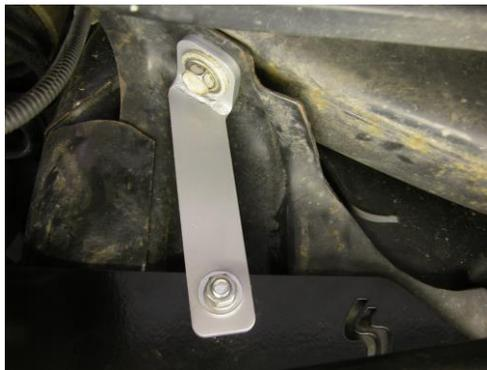
**Step 9:** Use the remaining two carriage head bolts, flat washers, lock washers, and nuts to attach the gas tank skid plate to your Skid Row Offroad transfer case skid plate as shown below.
